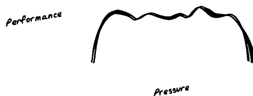
FIGURE 11-2. There is a limit to the value of pressure in increasing performance.
